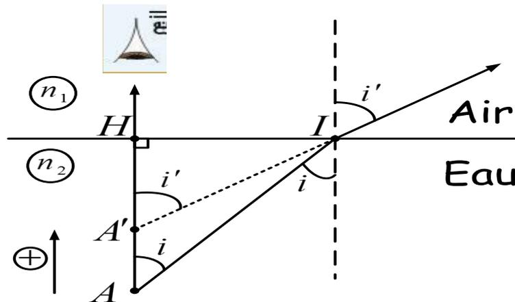
$$\operatorname{tg} i = \frac{\overline{HI}}{\overline{AH}} \quad \text{et} \quad \operatorname{tg} i' = \frac{\overline{HI}}{\overline{A'H}}$$
