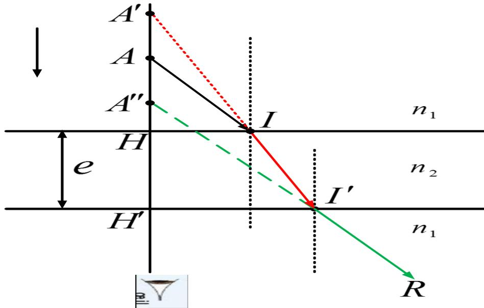
$$\left. \begin{array}{l} \frac{\overline{AH}}{n_1} = \frac{\overline{A'H}}{n_2} \\ \frac{\overline{A'H'}}{n_2} = \frac{\overline{A''H}}{n_1} \end{array} \right\} \Rightarrow \overline{AA''} = \overline{AH} + \overline{HH'} + \overline{H'A''} = \frac{n_1}{n_2} \overline{A'H} + e - \frac{n_1}{n_2} \overline{A'H'}$$
